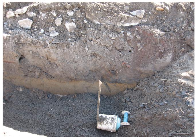
**Photo 6 - View at trenchwall materials NE of cofferdams; note: top of gravelly fill below surface soil contact with dredged fill.**
